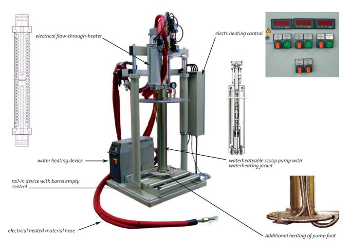
• The heating capacity of the water-heated pump enables a processing of most 1 component lamination glues directly at environmental temperature, WITHOUT, thus saving both the costs and extra time needed to pre-heat the barrel. An optional water-heated heating coil in the suction area of the pump as well as an electrically heated flowthrough heater enables material temperatures of up to 95 °C.
