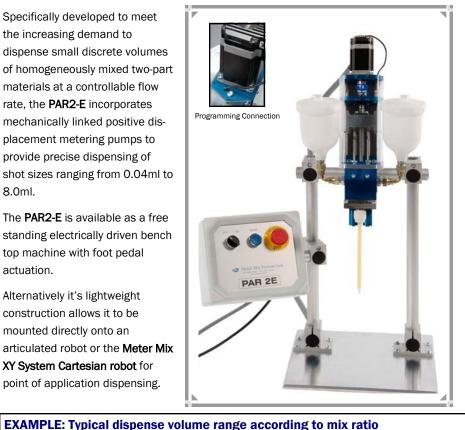
An extensive range of metering pump sizes and low volume disposable static mixing nozzles ensures that the PAR2-E can be tailored to suit most application requirements handling material mix ratios from 1:1 to 18:1.
