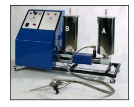
**Metering Pumps:** Single acting positive displacement.
