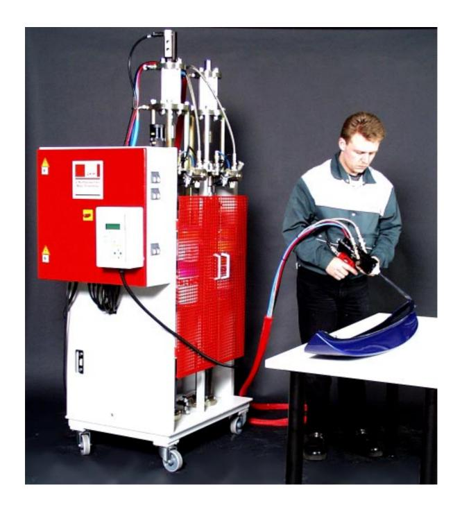
Metering Unit for Processing of Adhesives PolyMix 9020 / 9220
