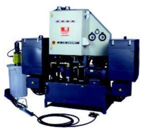
Downdraught Heaters 6.5 kW downdraught heaters are used to pre-heat the components during the suction phase. The temperature can be steplessly set up to 100 C.
